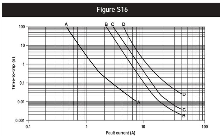
Figures S11–S18. Typical Time-to-Trip Curves at 20°C for Surface-mount Devices
