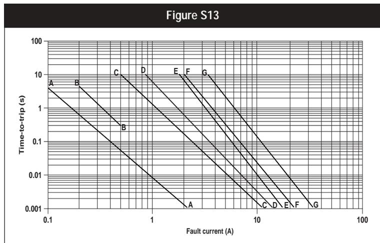
Figures S11–S18. Typical Time-to-trip Curves at 20°C for Surface-mount Devices *continued*
