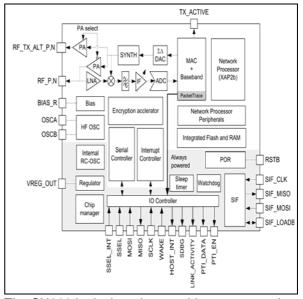
The SN260 is designed to provide customers the flexibility of choosing their own microcontroller to run their application, while interfacing to the SN260 to provide all the ZigBee functionality. This flexibility allows customers to ZigBee-enable existing products very rapidly using toolchains that they are familiar with.
