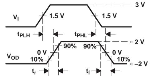
Figure 4. Driver Switching Test Circuit and Voltage Waveforms
