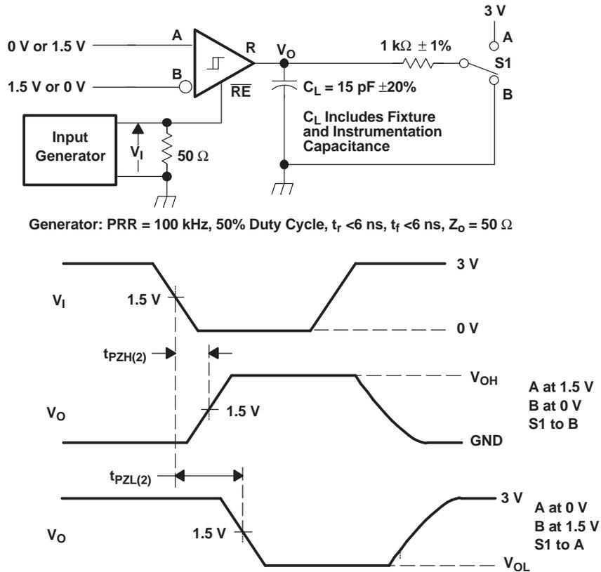
Figure 10. Receiver Enable Time From Standby (Driver Disabled)
