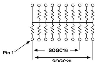
15 or 19 resistors with one pin common
