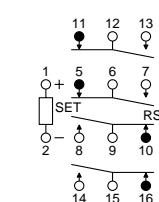
Diagram shows the "reset" position when terminals 3 and 4 are energized. Energize terminals 1 and 2 to transfer contacts.
