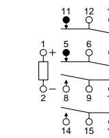
**PC board pattern (Bottom view)**
