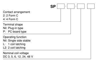
Notes: 1. PC board type and 1 coil latching type are manufactured by lot upon receipt of order.
