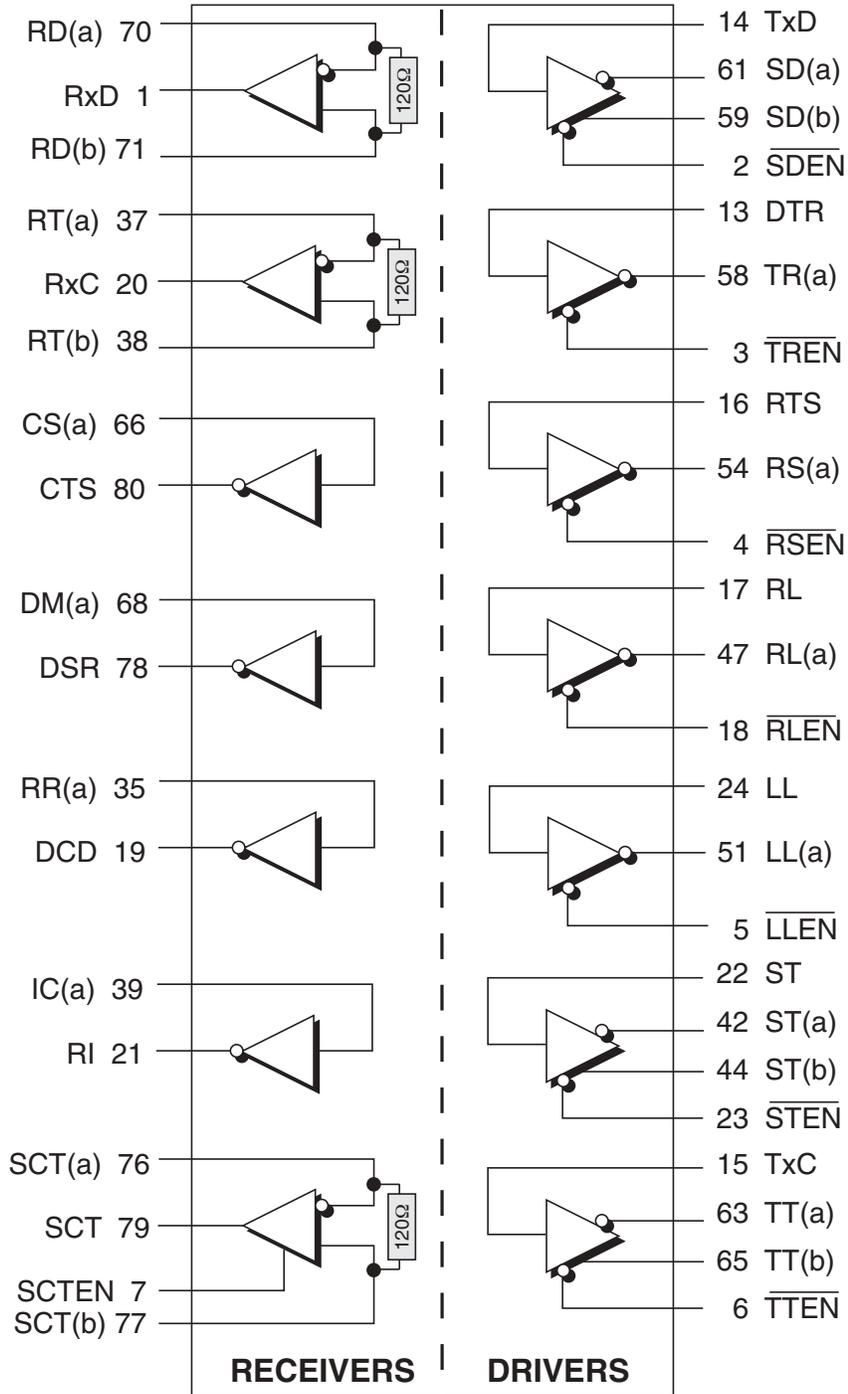
Figure 60. Mode Diagram — V.36
