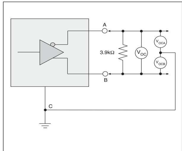
Figure 16. V.11 and V.35 Driver Output Open-Circuit Voltage
