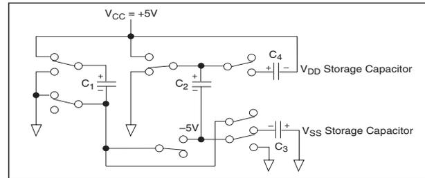
Figure 48. Charge Pump Phase 2 for  $\pm 5V$ .
