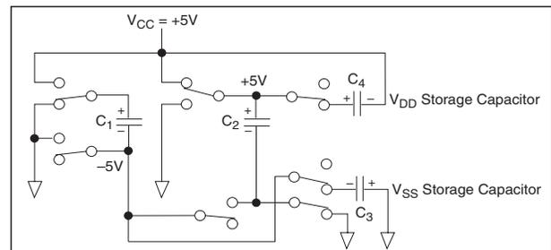
Figure 46. Charge Pump Phase 1 for  $\pm 5V$ .
