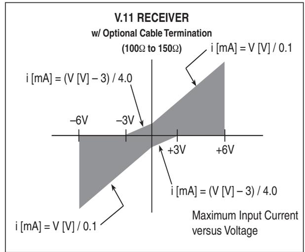
Figure 24. V.11 Receiver Input Graph w/ Termination
