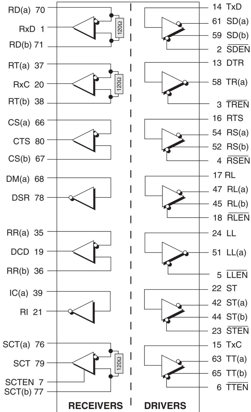
Figure 59. Mode Diagram — EIA-530A
