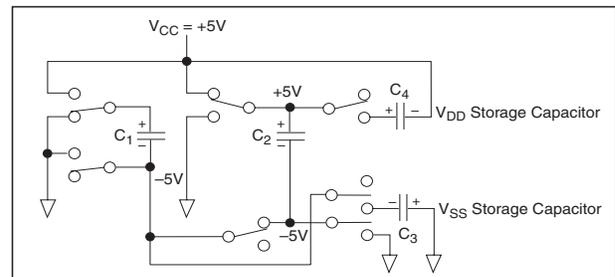
Figure 45. Charge Pump Phase 1 for  $\pm 10V$ .
