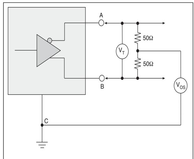
Figure 25. V.35 Driver Output Test Terminated Voltage
