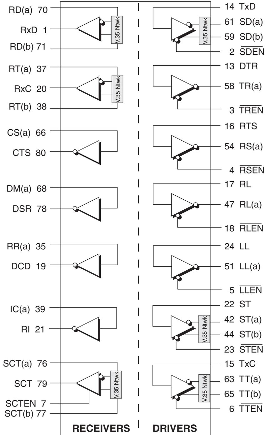
Figure 54. Mode Diagram — V.35
