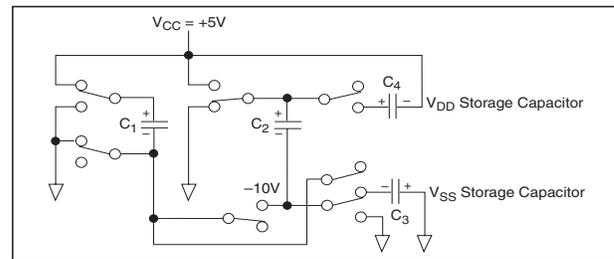
Figure 47. Charge Pump Phase 2 for  $\pm 10V$ .
