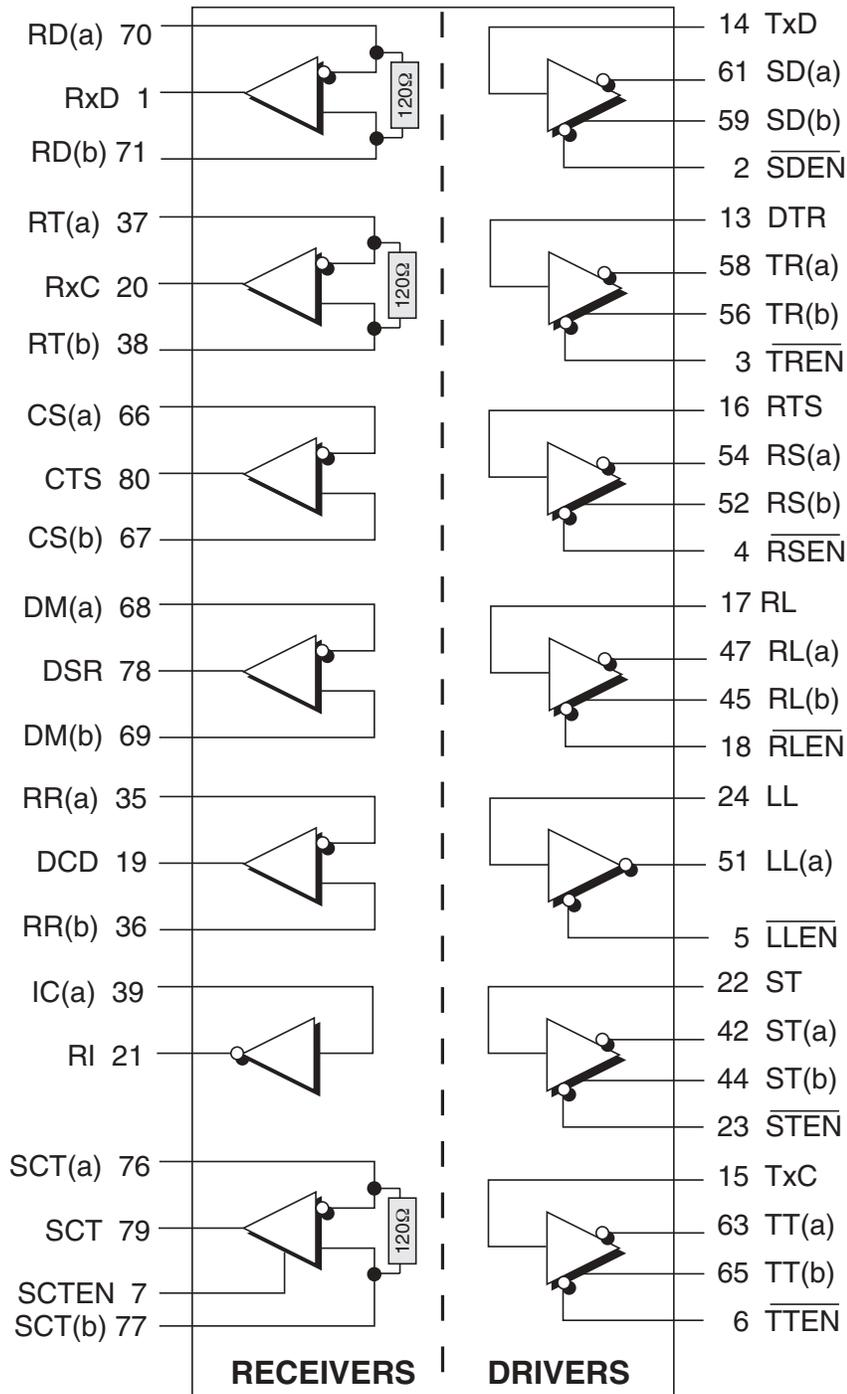
Figure 58. Mode Diagram — EIA-530
