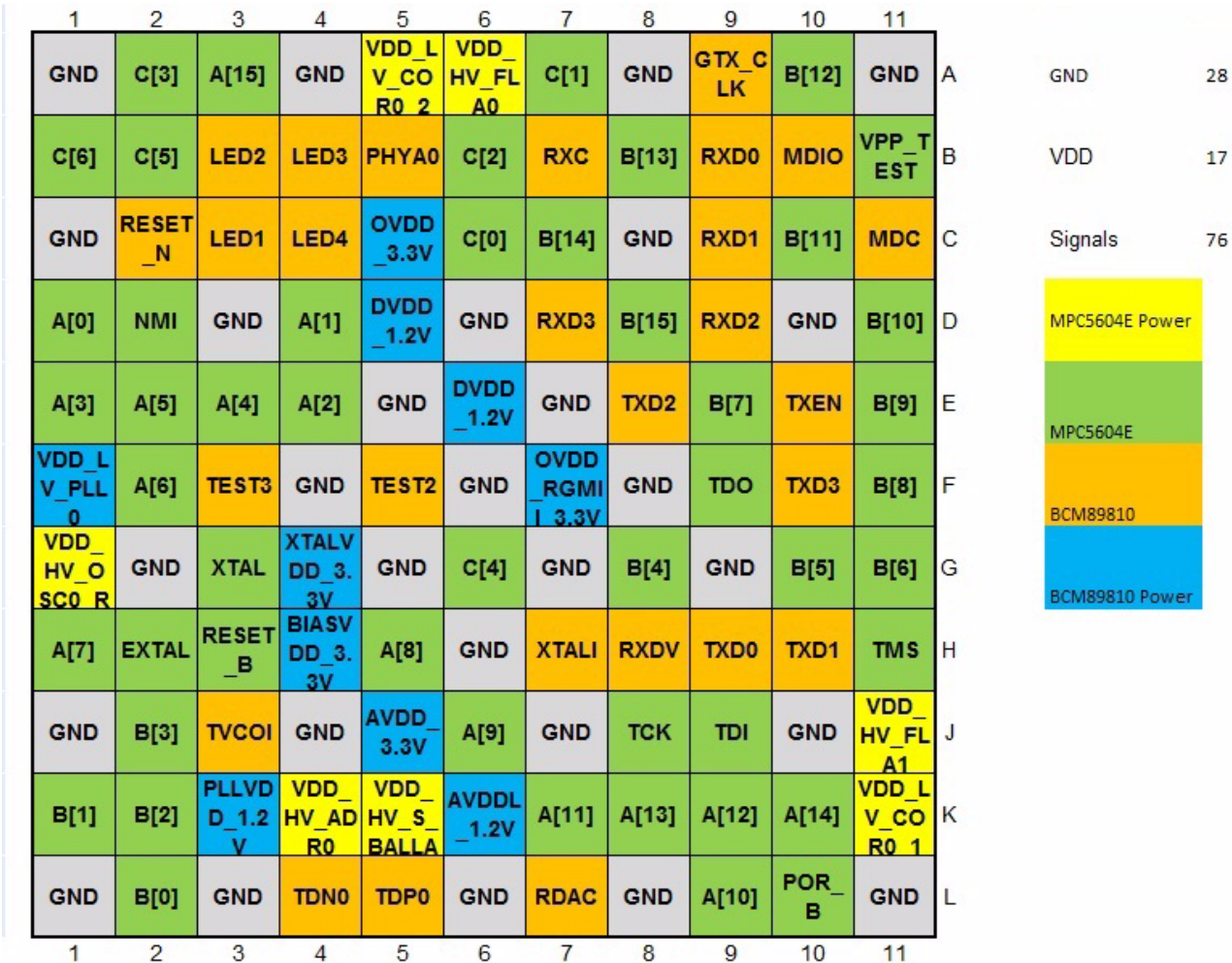
Figure 2. 121 MAPBGA pinout(top view)
