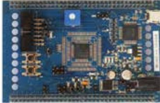
SPC56D-Discovery with SPC560D40L1 order code: SPC560D-DIS
