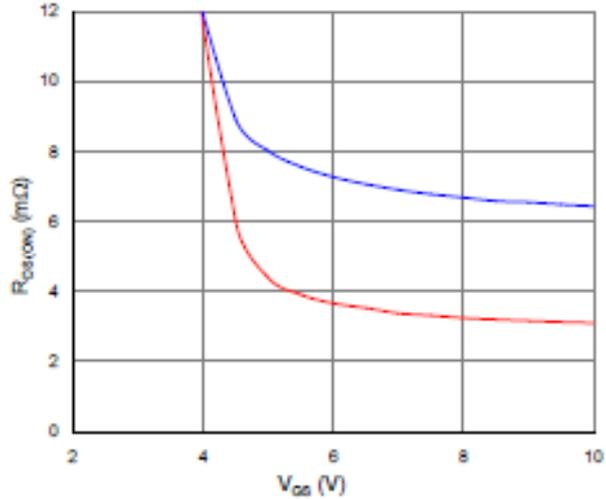
Fig. 8 On Resistance vs Gate Source Voltage
