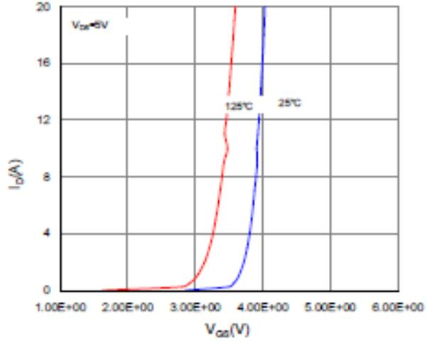
Fig. 2 Transfer Characteristics
