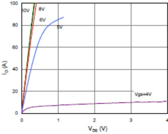
Fig. 1 Output Characteristics
