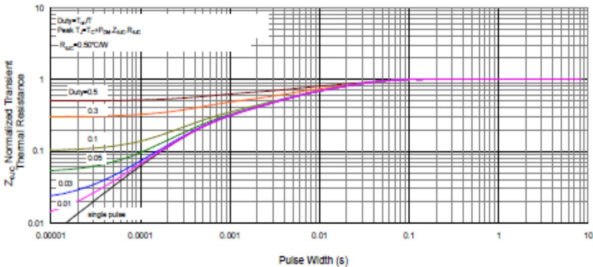
Fig. 9 Normalized Thermal Transient Impedance, Junction to Foot
