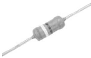
A multi layer metal film is deposited on a high grade ceramic body. After a helical groove has been cut in the resistive layer, tinned electrolytic copper wires are welded to the end-caps. The resistors are coated with a light blue non-flammable lacquer, which provides electrical, mechanical, and climatic protection.
