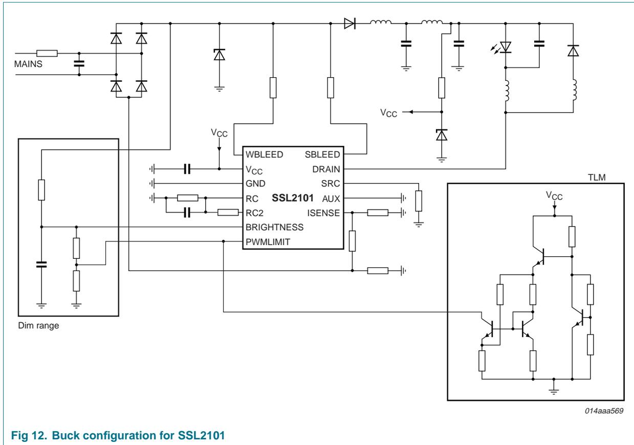
**Fig 12. Buck configuration for SSL2101**
