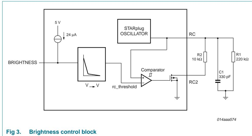
Fig 3. Brightness control block
