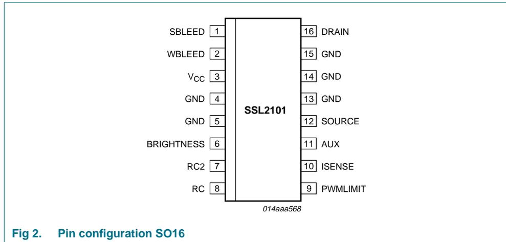
Fig 2. Pin configuration SO16
