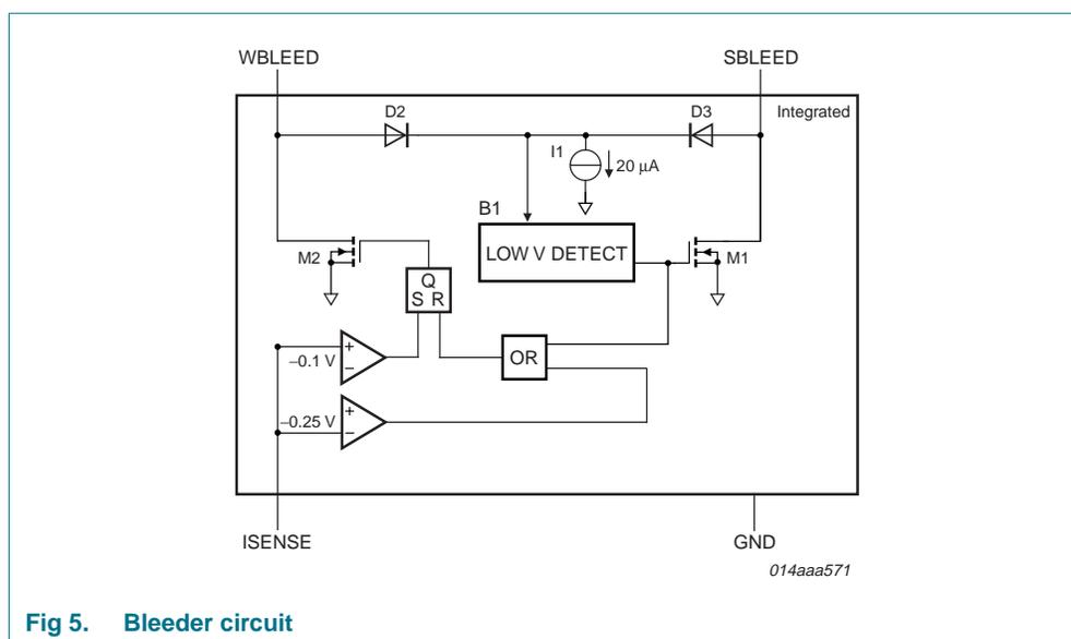
Fig 5. Bleeder circuit
