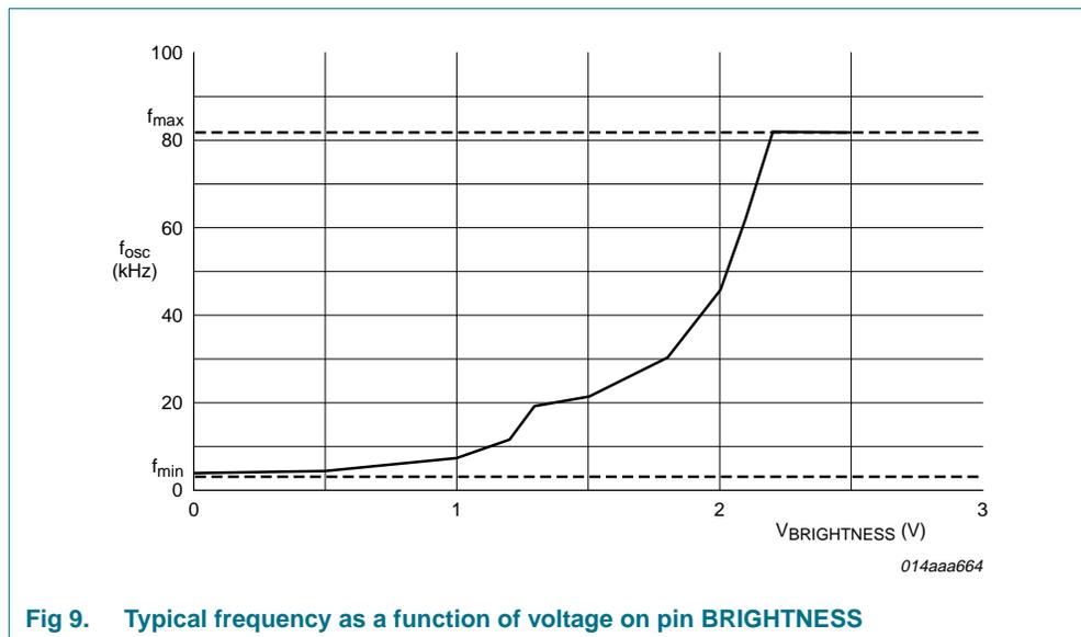
**Fig 9. Typical frequency as a function of voltage on pin BRIGHTNESS**
