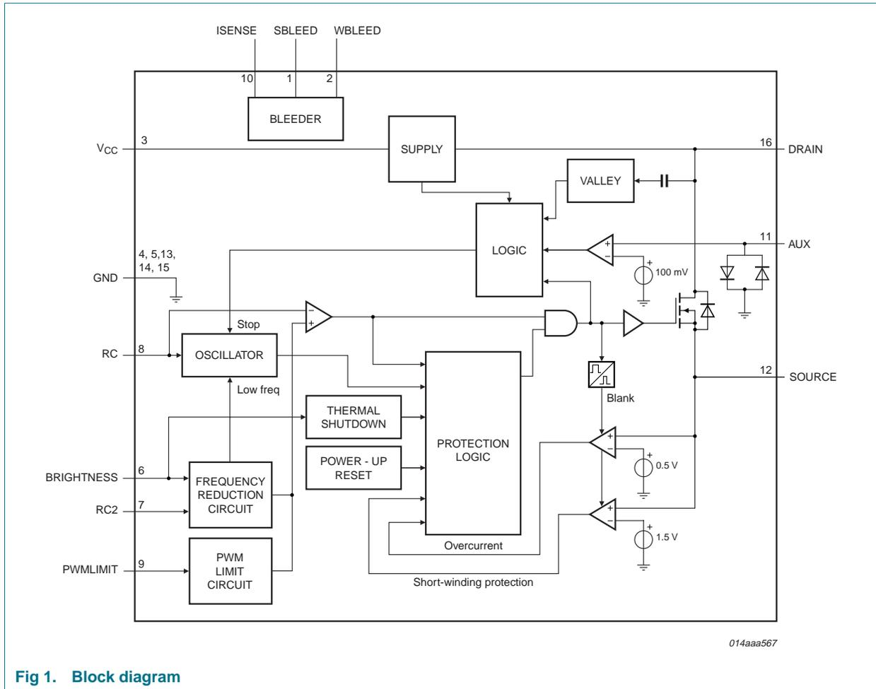
Fig 1. Block diagram
