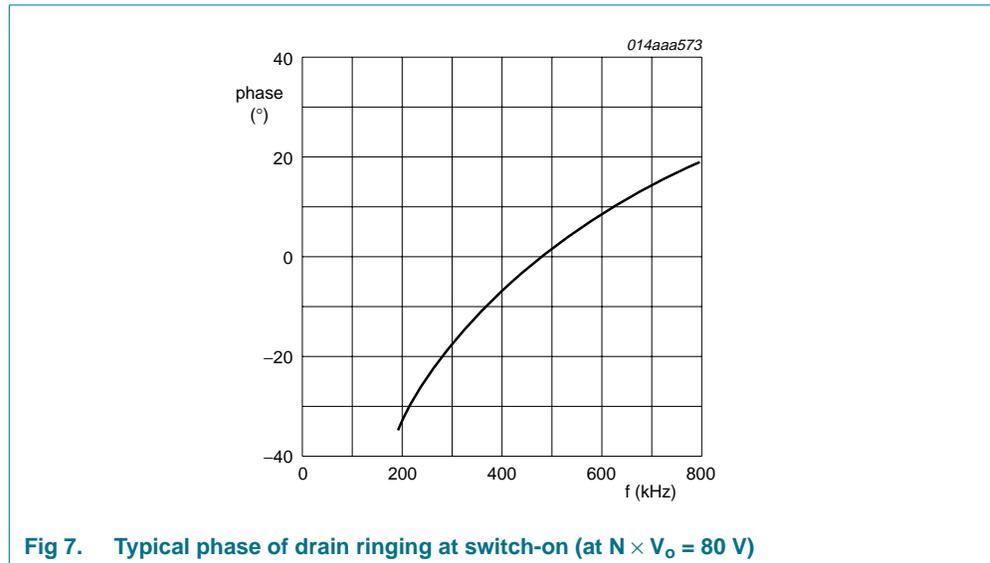
Fig 7. Typical phase of drain ringing at switch-on (at  $N \times V_o = 80 \text{ V}$ )
