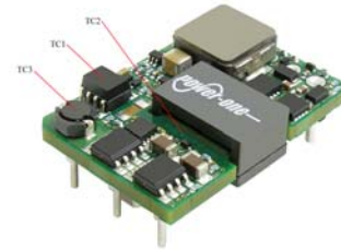
Fig. H: Locations of the thermocouple for thermal testing.
