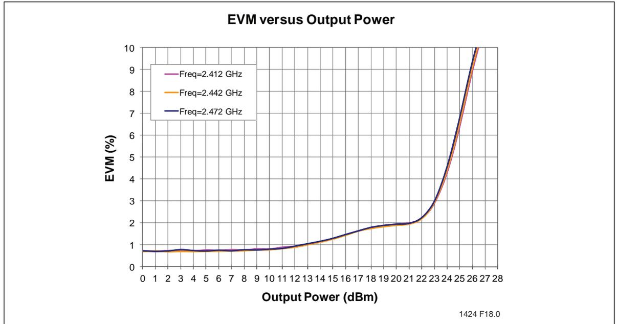
**Figure 12:** EVM versus Output Power measured with equalizer training set to sequence only
