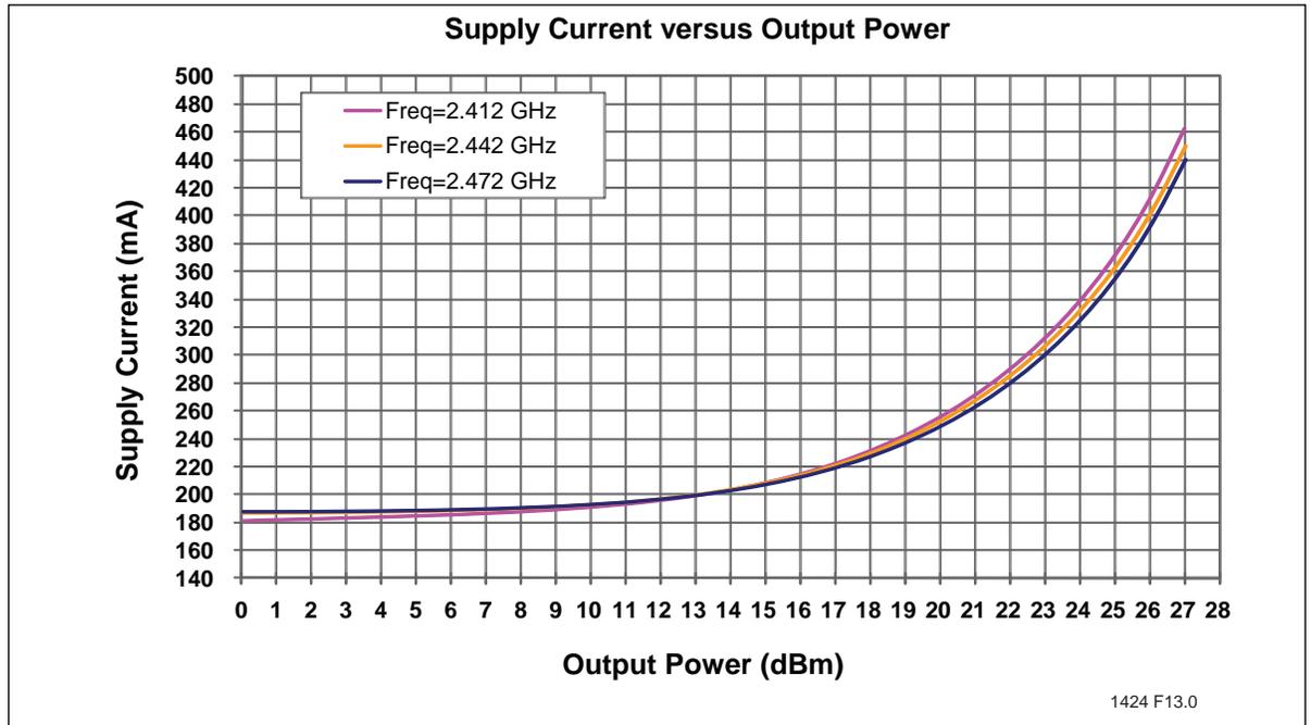
**Figure 8:** Total Current Consumption for 802.11g operation versus Output Power
