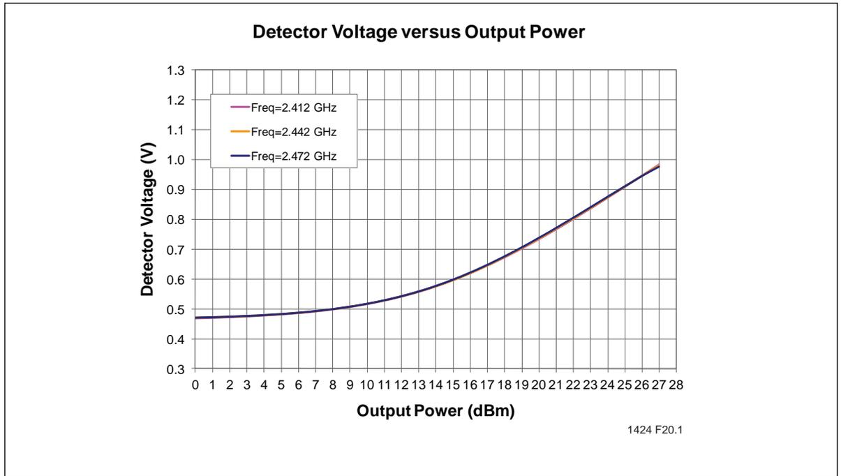
**Figure 15:**Detector Characteristics versus Output Power
