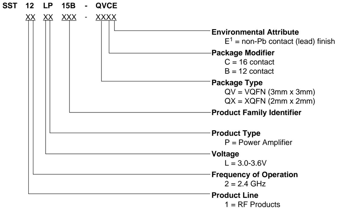
1. Environmental suffix "E" denotes non-Pb solder. SST non-Pb solder devices are "RoHS Compliant".
