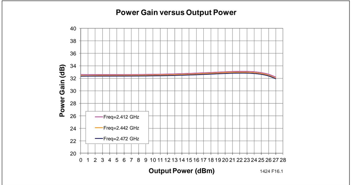
Figure 13: Gain versus Output Power
