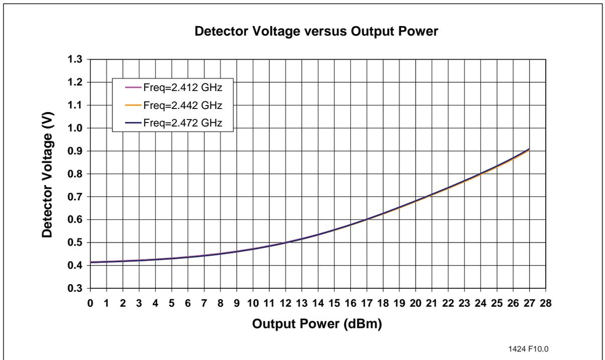
**Figure 21:**Detector Characteristics versus Output Power
