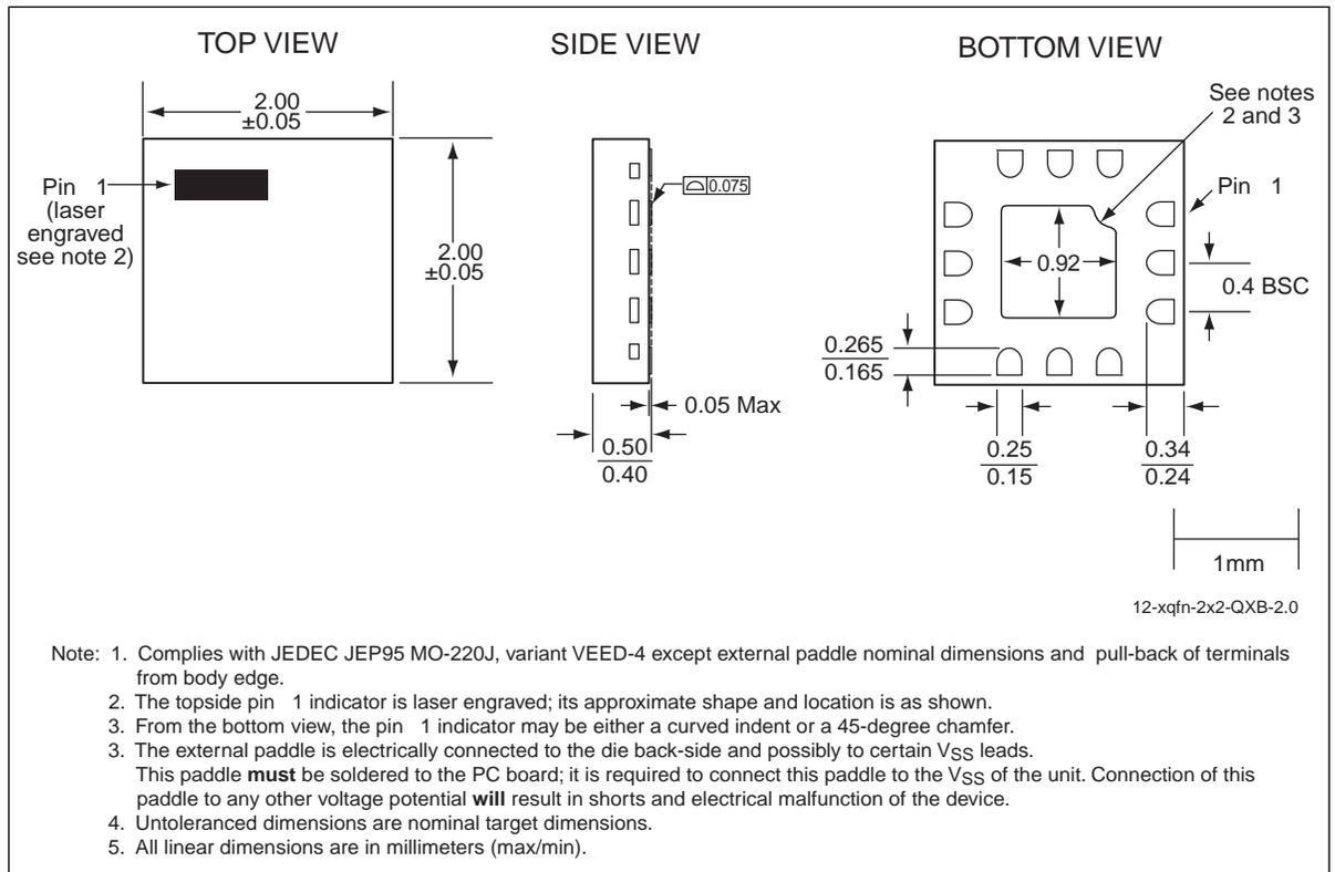
**Figure 24:** 12-contact Extremely-thin Quad Flat No-lead (XQFN)
