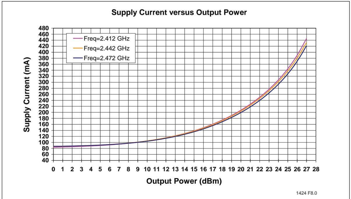
**Figure 20:**Total Current Consumption for 802.11g operation versus Output Power
