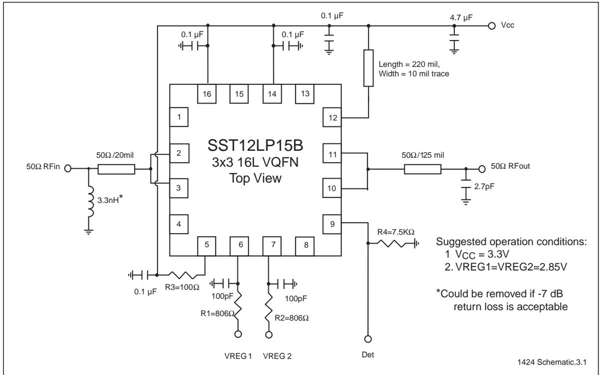
**Figure 22:** Typical Schematic for High-Linearity 802.11b/g/n Applications for 16-contact VQFN
