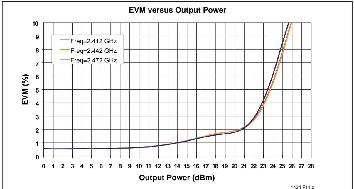
Figure 6: EVM versus Output Power measured with equalizer training set to sequence only
