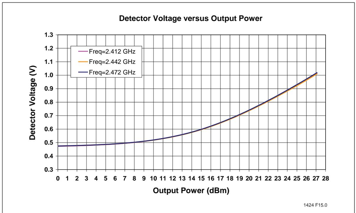
**Figure 9:** Detector Characteristics versus Output Power
