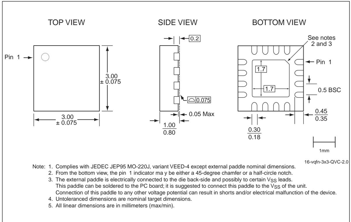
**Figure 23:** 16-contact Very-thin Quad Flat No-lead (VQFN)
