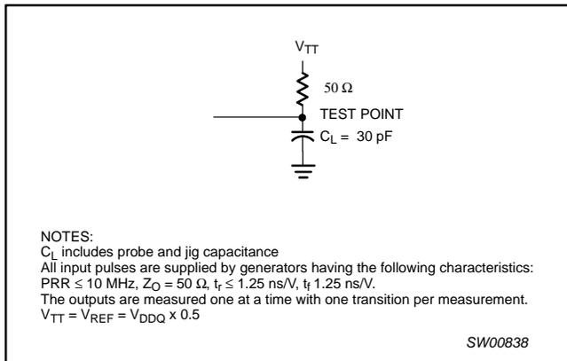
Figure 1. Load circuitry
