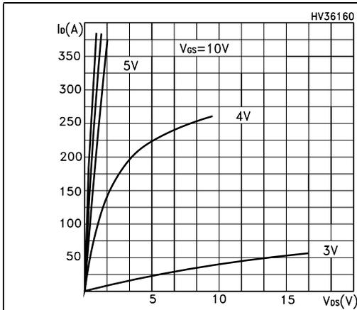
Figure 5. Transfer characteristics
