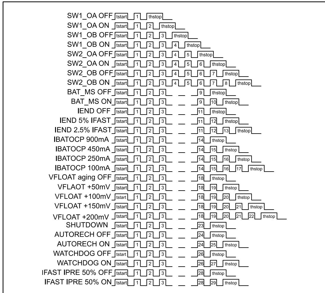
Figure 21: Single wire programming (SW_SEL INPUT)
