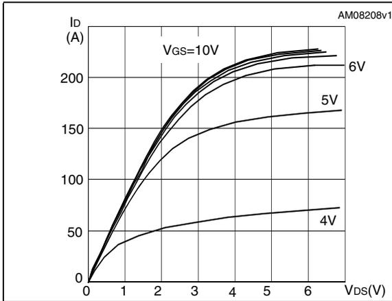
Figure 5. Transfer characteristics
