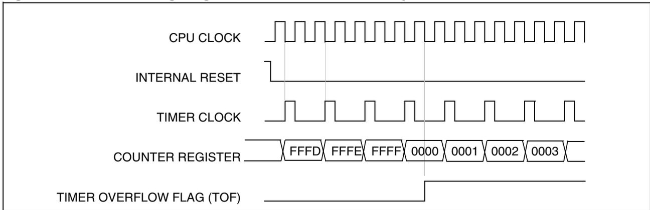
Figure 37. Counter Timing Diagram, internal clock divided by 4
