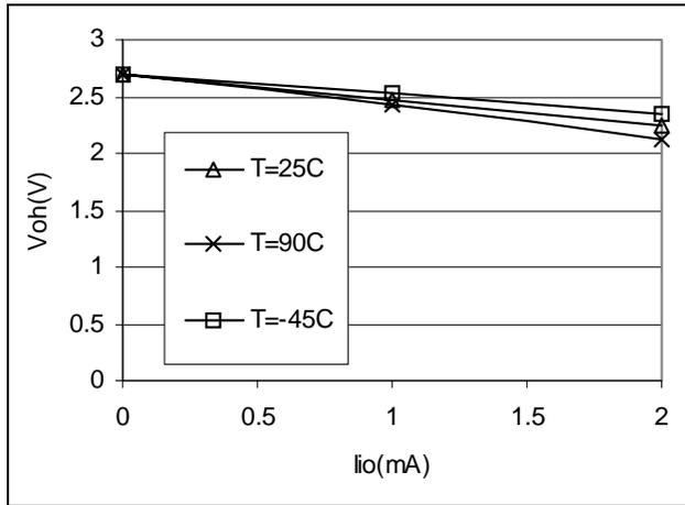
Figure 86. Typ.  $V_{OH}$  at  $V_{DD}=3V$
