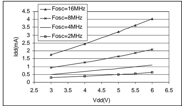
Figure 67. Typical  $I_{DD}$  in SLOW at  $T_A=25^\circ\text{C}$
