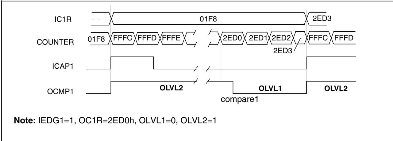
Figure 45. Pulse Width Modulation Mode Timing Example
