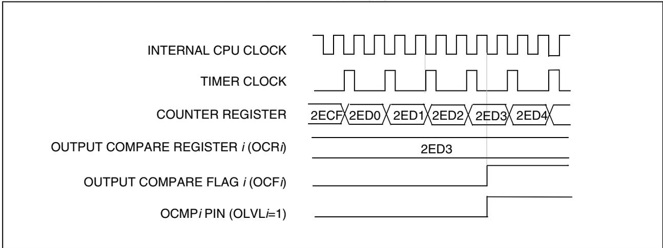
Figure 43. Output Compare Timing Diagram,  $f_{TIMER} = f_{CPU}/4$
