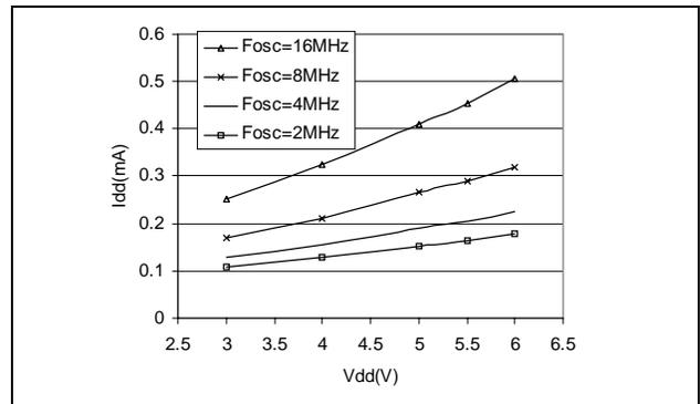
**SUPPLY CURRENT CHARACTERISTICS (Cont'd)****13.4.2 HALT and ACTIVE-HALT Modes**
