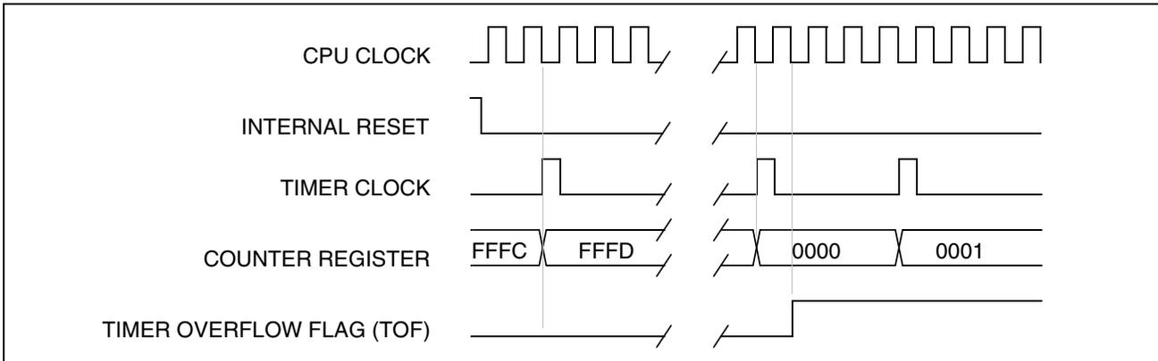
Figure 38. Counter Timing Diagram, internal clock divided by 8
