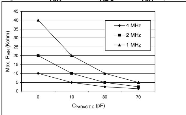
Figure 98. Recommended C<sub>AIN</sub>/R<sub>AIN</sub> values<sup>3)</sup>
