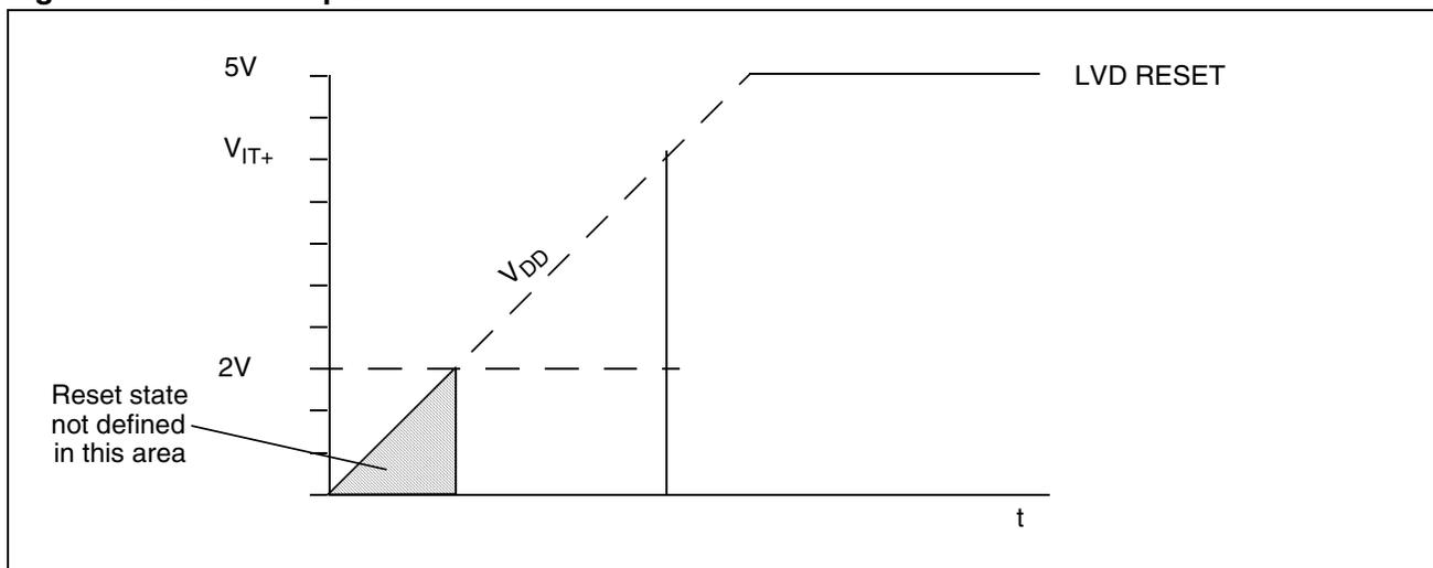
**Note:** When the LVD is enabled, the MCU reaches its authorized operating voltage from a reset state. However, in some devices, the reset signal may be undefined until  $V_{DD}$  is approximately 2V. As a consequence, the I/Os may toggle when  $V_{DD}$  is below this voltage.
