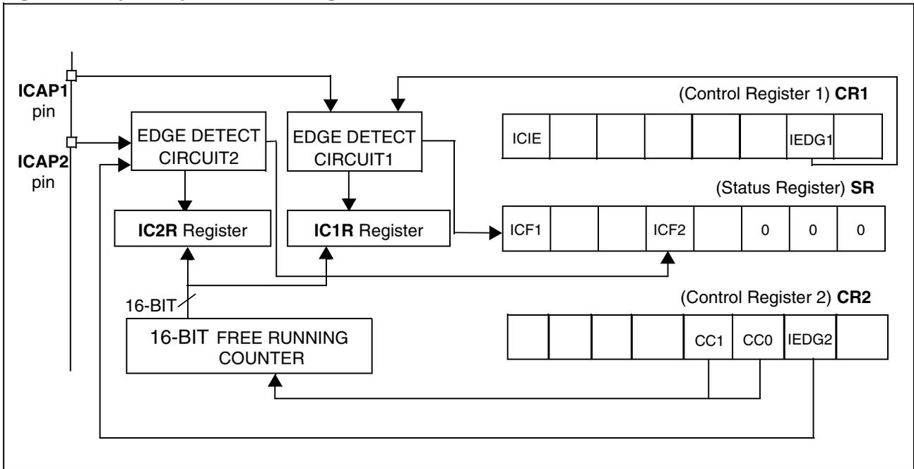
Figure 40. Input Capture Timing Diagram
