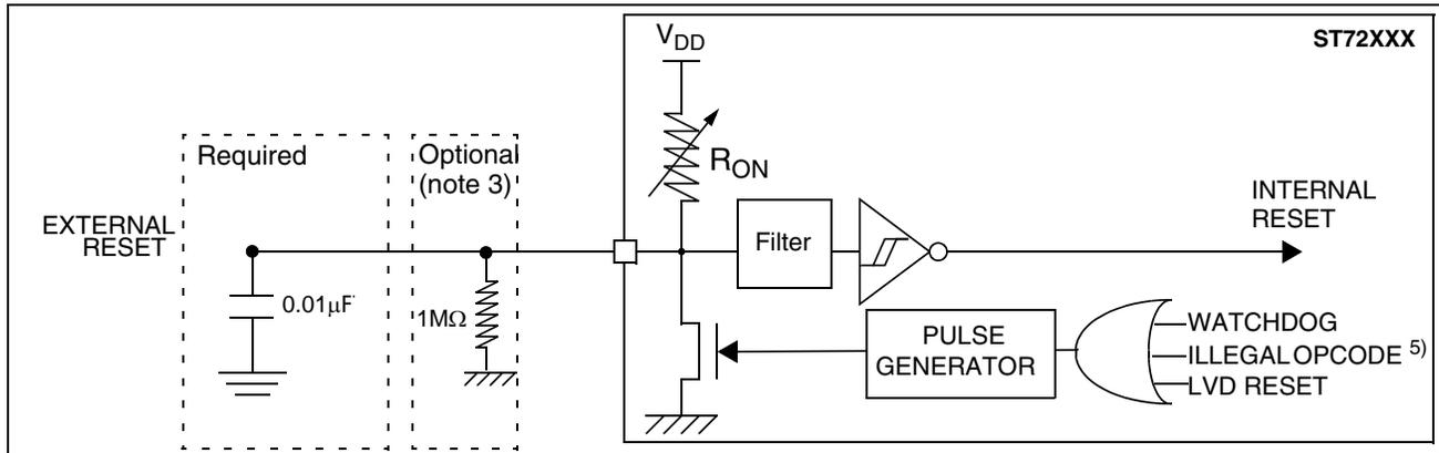
Figure 92.  $\overline{\text{RESET}}$  pin protection when LVD is disabled.<sup>1)</sup>
