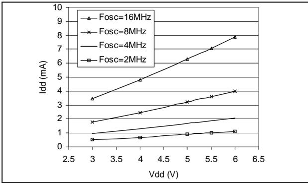
Figure 68. Typical  $I_{DD}$  in WAIT at  $T_A=25^\circ\text{C}$
