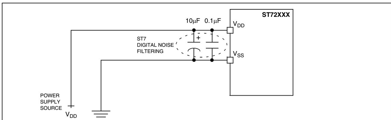
1. The suggested 10µF and 0.1µF decoupling capacitors on the power supply lines are proposed as a good price vs. EMC performance tradeoff. They have to be put as close as possible to the device power supply pins. Other EMC recommendations are given in AN1709.
