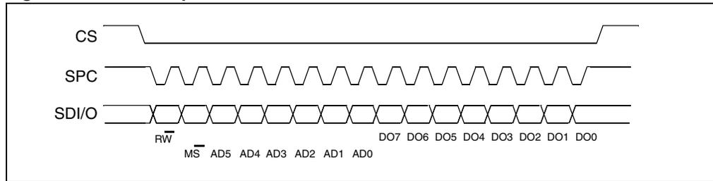
The SPI Read command is performed with 16 clock pulses:
