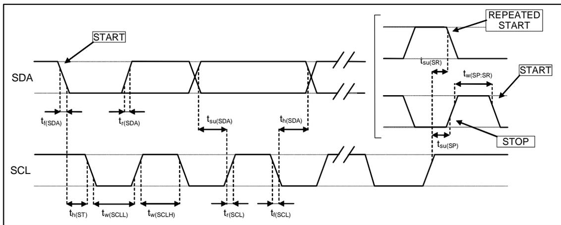
4. Measurement points are done at 0.2·V<sub>dd\_IO</sub> and 0.8·V<sub>dd\_IO</sub>, for both ports
