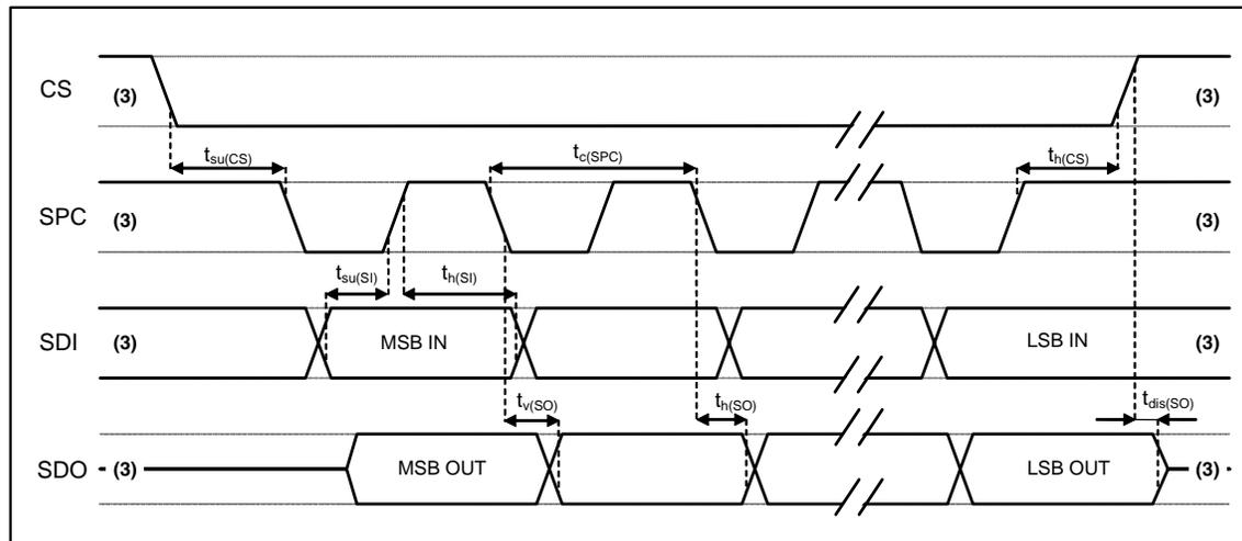
2. Measurement points are done at 0.2·V<sub>dd\_IO</sub> and 0.8·V<sub>dd\_IO</sub>, for both Input and Output port
