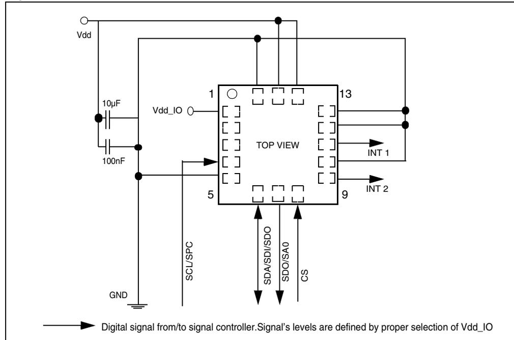
The device core is supplied through Vdd line while the I/O pads are supplied through Vdd\_IO line. Power supply decoupling capacitors (100 nF ceramic, 10 µF Al) should be placed as near as possible to the pin 14 of the device (common design practice).
