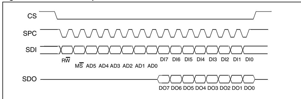
**CS** is the Serial Port Enable and it is controlled by the SPI master. It goes low at the start of the transmission and goes back high at the end. **SPC** is the Serial Port Clock and it is controlled by the SPI master. It is stopped high when **CS** is high (no transmission). **SDI** and **SDO** are respectively the Serial Port Data Input and Output. Those lines are driven at the falling edge of **SPC** and should be captured at the rising edge of **SPC**.
