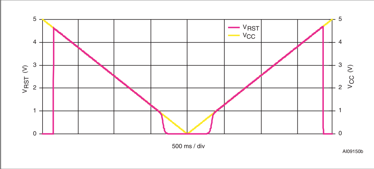
Figure 21. RST output voltage vs. supply voltage
