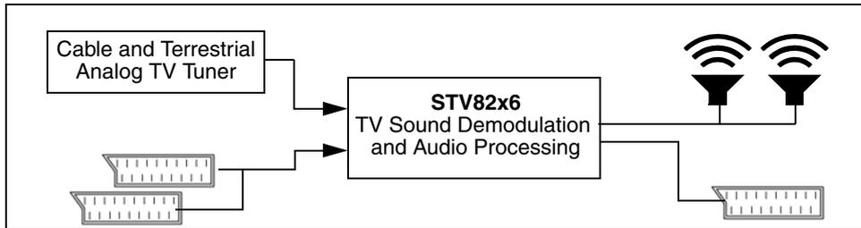
Figure 3: Typical Application with Subwoofer and Headphone
