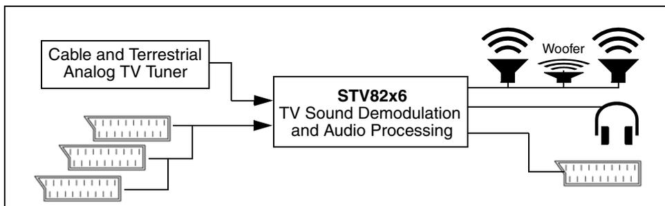
Figure 4: Typical Application Electrical Diagram for STV82x6 in SDIP56 package
