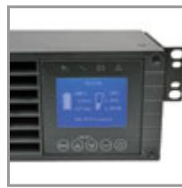
High-performance on-line double-conversion UPS with interactive LCD interface ideal for any critical voice, data, medical or industrial IT application. Converts AC input to DC and then fully regulated sine wave AC power.
