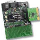
An easy-to-use ZigBee™ Technology wireless communication protocol development and demonstration platform. The kit includes the ZigBee protocol stack and two PICDEM Z boards, each with an RF daughter card. The demonstration board is also equipped with a 6-pin modular connector to interface directly with MPLAB® ICD 2.
