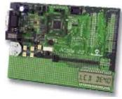
Demonstrates the main features of the LCD Flash 28-, 40-, 64- and 80-pin PIC® microcontrollers with power management features. The board is populated with the PIC18F8490 and other devices are supported via a transition socket. A sample LCD glass display is included for custom prototyping. The PICDEM LCD kit provides tutorial firmware, which is included in the preprogrammed devices.
