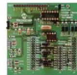
Evaluates and demonstrates the MCP2122 or MCP2120 IrDA® Standard Encoder/Decoder devices. A header allows the MCP212X Daughter Board to be easily jumpered into systems for development purposes. This board also interfaces with these new low-cost PIC®
