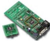
This low-cost demo board is used to evaluate the performance of high-end 8-bit PIC18F series. The board features a PIC18F8722 microcontroller, which is the superset of the entire 64- and 80-pin PIC18FXXX general purpose family. A daughter board (mezzanine) is also part of the kit and allows different processors sharing the same pin out to be mounted and tested on the explorer board.
