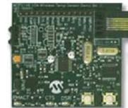
Demonstrates the MCP2140 device in a real-world application. This design is an example of how to integrate an IrDA standard port into a system.
