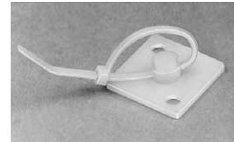
\*The rubber-based adhesive backing on these mounts has a tensile strength of 6 lbs. [26.7 N] per square inch. This rating applies in temperatures from -50°F [-45°C] to 180°F [82°C]. For best performance, mounts should be applied to a smooth, clean, dry, and oil-free surface.
