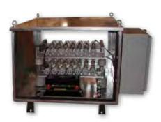
Neutral-Grounding Resistors (NGRs) are used to ground power systems by inserting a resistor between the system neutral and ground. This lowers the prospective ground-fault current to a predetermined value. Because the system is grounded, transient overvoltages do not occur and ground-fault current can flow, allowing it to be detected and measured.
