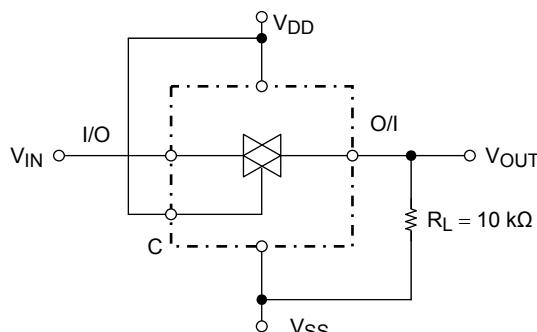
$$R_{ON} = 10 \times \frac{(V_{IN} - V_{OUT})}{V_{OUT}} \text{ [k}\Omega\text{]}$$
