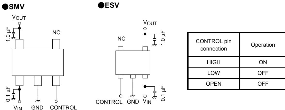
The figure above shows the recommended configuration for using a Low-Dropout regulator. Insert a capacitor at VOUT and VIN pins for stable input/output operation. (Ceramic capacitors can be used).
