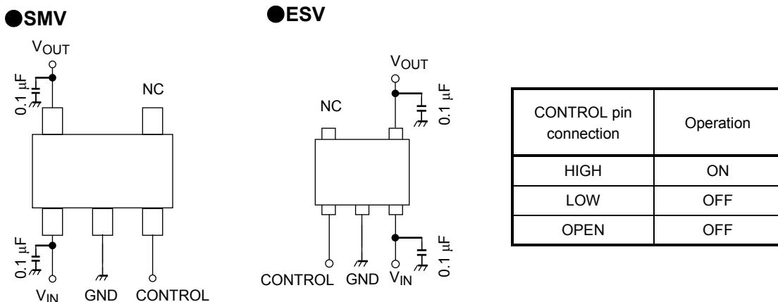
The figure above shows the recommended configuration for using a Low-Dropout regulator. Insert a capacitor at V<sub>OUT</sub> and V<sub>IN</sub> pins for stable input/output operation. (Ceramic capacitors can be used).
