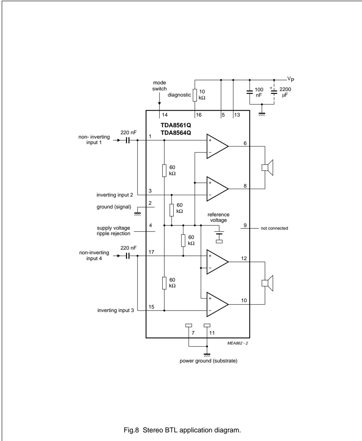
Fig.8 Stereo BTL application diagram.
