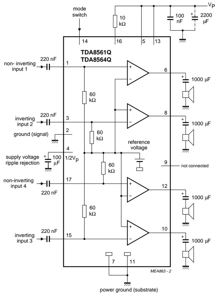
Fig.9 Quad single-ended application diagram 1.
