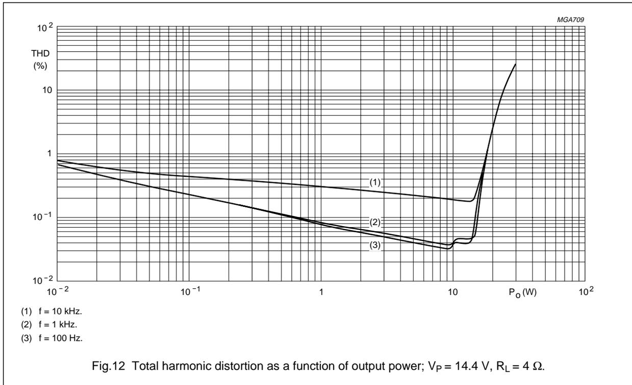
Fig.12 Total harmonic distortion as a function of output power;  $V_P = 14.4 \text{ V}$ ,  $R_L = 4 \Omega$ .
