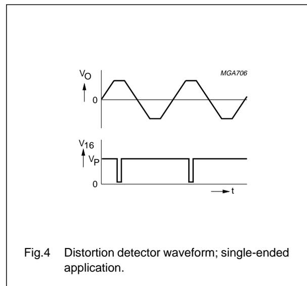
Fig.4 Distortion detector waveform; single-ended application.
