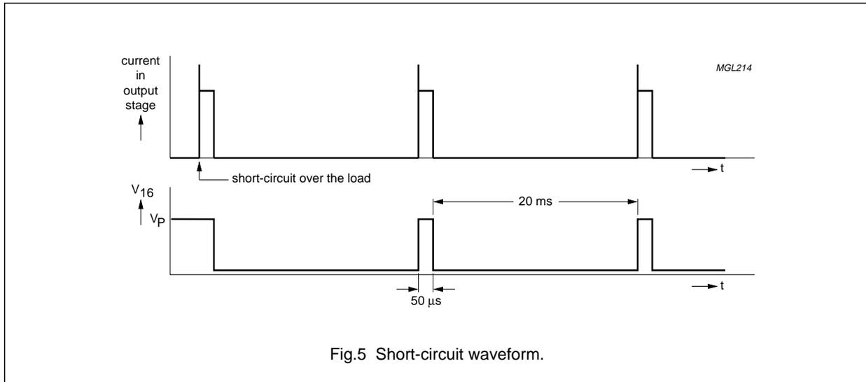
Fig.5 Short-circuit waveform.
