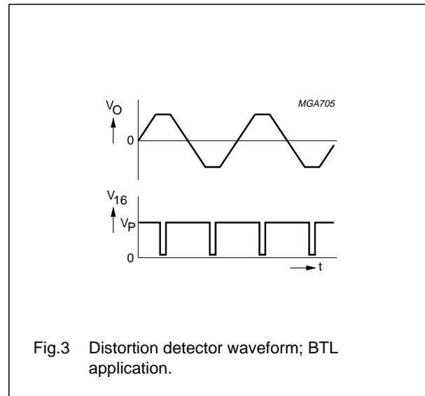
Fig.3 Distortion detector waveform; BTL application.
