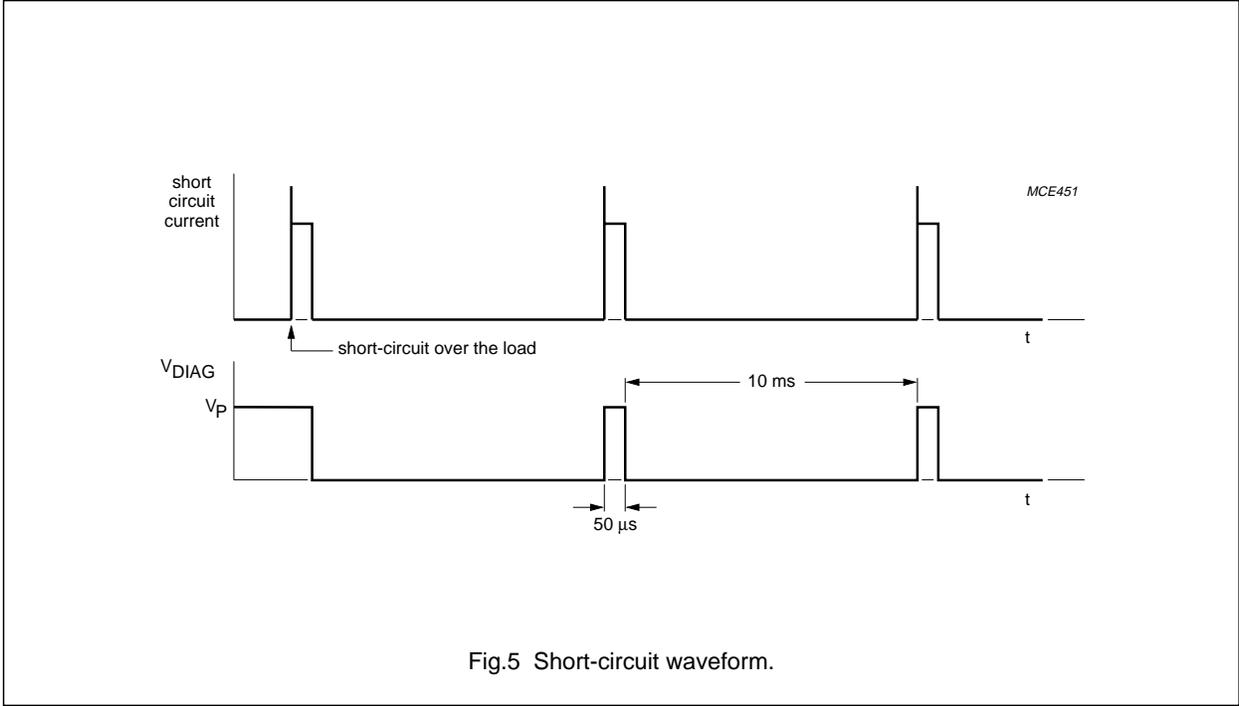
Fig.5 Short-circuit waveform.
