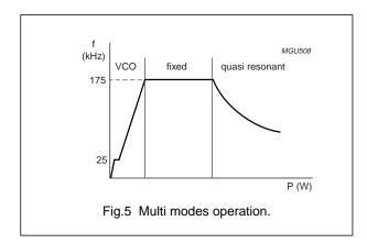
The next converter stroke is started only after demagnetization of the transformer current (zero current switching), while the drain voltage has reached the lowest voltage to prevent switching losses (green function). The primary resonant circuit of the primary inductance and drain capacitor ensures this quasi-resonant operation. The design can be optimized in such a way that zero voltage switching can be reached over almost the universal mains range.
