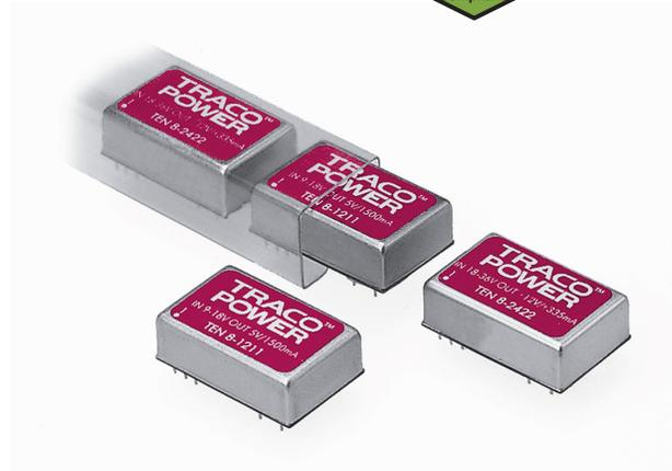
The TEN 8 series is a family of high performance 8 W DC/DC converter modules featuring wide 2:1 input voltage ranges in a DIP-24 package with industry standard footprint. A very high efficiency allows an operating temperature range of -40°C to +85°C. A built-in EMI input filter complies with EN 55022, class A without external components. Further standard features include remote On/Off and short-circuit protection.
