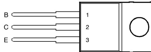
Pin 2 is in electrical contact with the mounting base.
