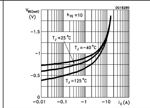
**Figure 10. Base-emitter on voltage for NPN type**
