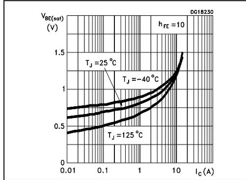
**Figure 9. Base-emitter saturation voltage for PNP type**
