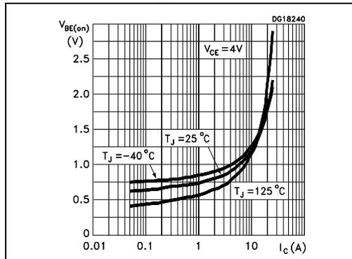
**Figure 11. Base-emitter on voltage for PNP type**
