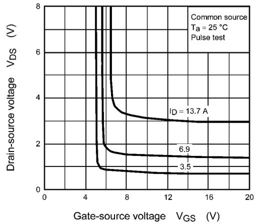
**Fig. 8.4  $V_{DS} - V_{GS}$**
