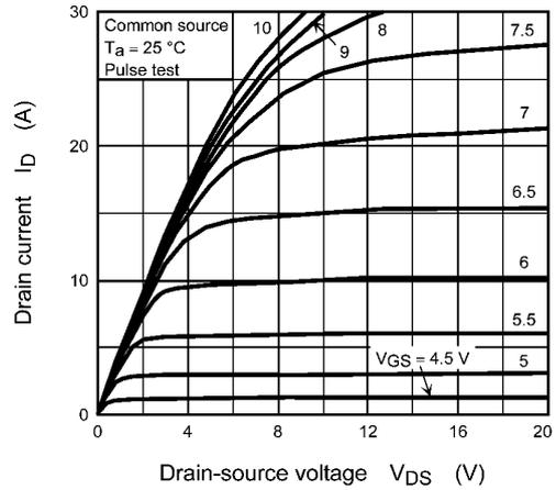
**Fig. 8.2  $I_D - V_{DS}$**
