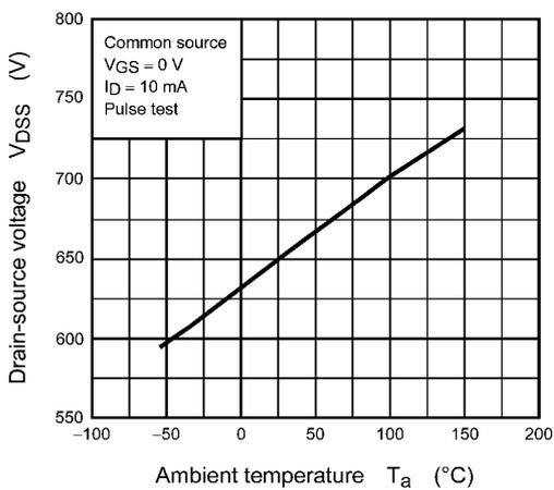
**Fig. 8.5  $V_{DSS} - T_a$**
