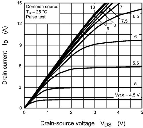
**Fig. 8.1  $I_D - V_{DS}$**
