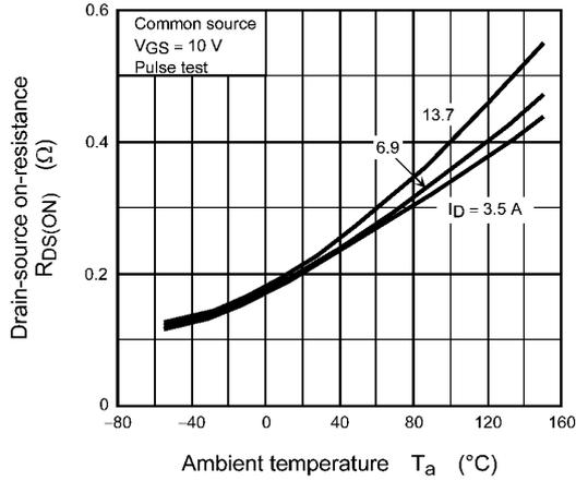
Fig. 8.7  $R_{DS(ON)} - T_a$
