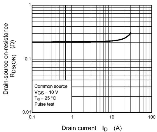
**Fig. 8.6  $R_{DS(ON)} - I_D$**
