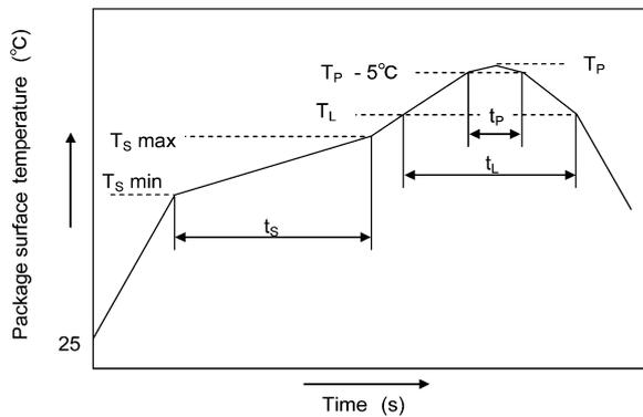
**Fig. 10.2.1 Temperature Profile for Lead(Pb)-free Soldering (example)**
