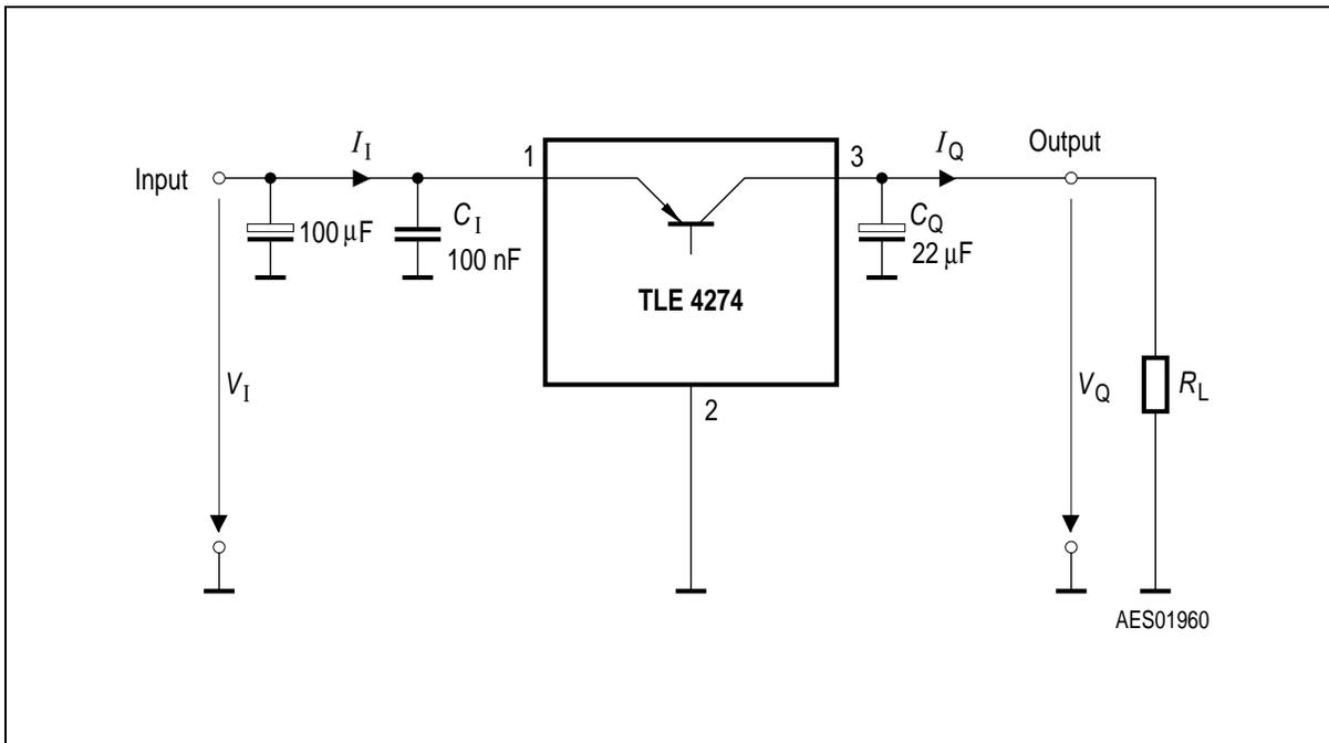
**Figure 3 Measuring Circuit**
