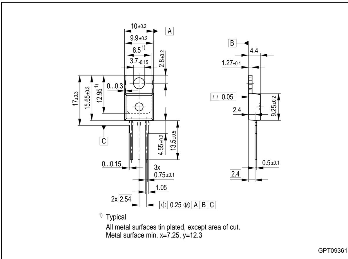
**Figure 5 PG-TO220-3-1 (Plastic Transistor Single Outline)**
