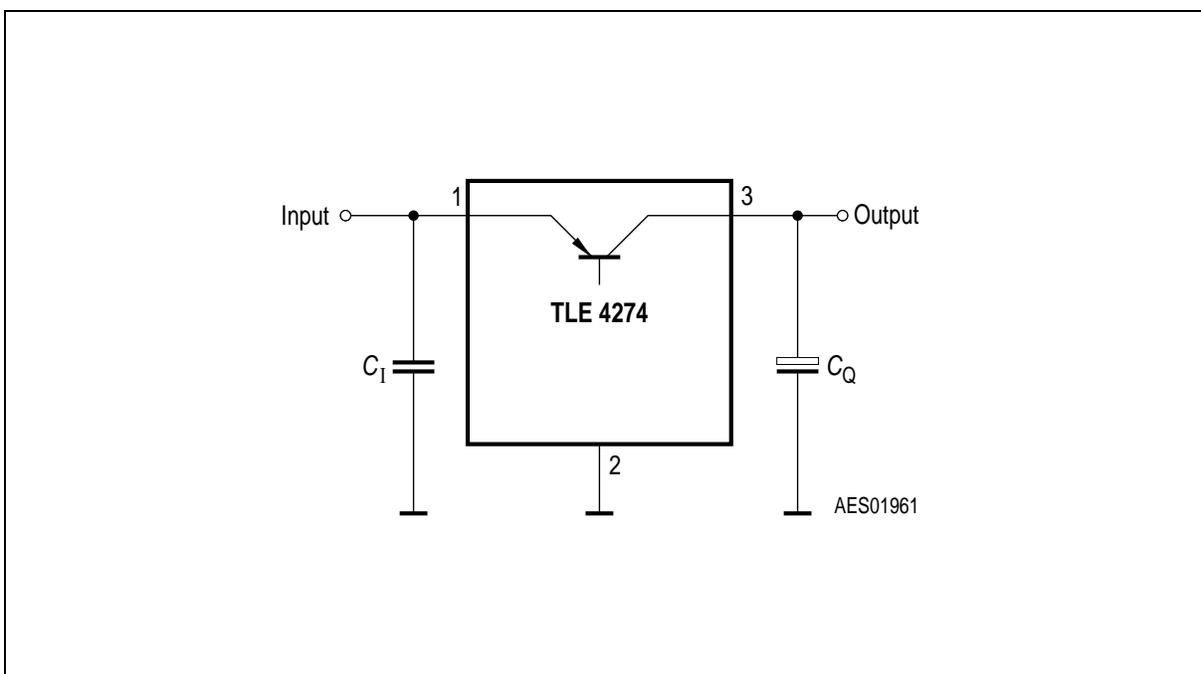
**Figure 4 Application Circuit**
