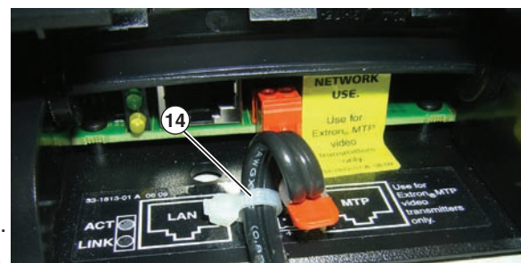
Figure 5. Securing the power cable
