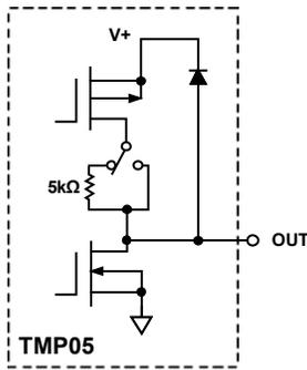
Figure 23. TMP05 One Shot Mode OUT Pin Configuration
