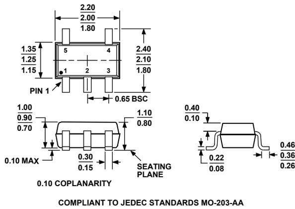
Figure 38. 5-Lead Thin Shrink Small Outline Transistor Package [SC-70] (KS-5)
