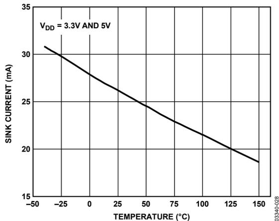
Figure 14. TMP06 Open Drain Sink Current vs. Temperature
