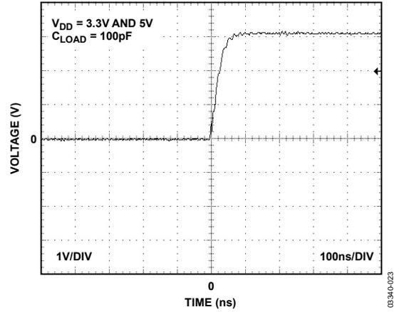
Figure 9. TMP05 Output Rise Time at 25°C
