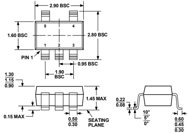
Figure 39. 5-Lead Small Outline Transistor Package [SOT-23] (RJ-5)
