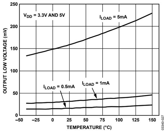
Figure 13. TMP06 Output Low Voltage vs. Temperature
