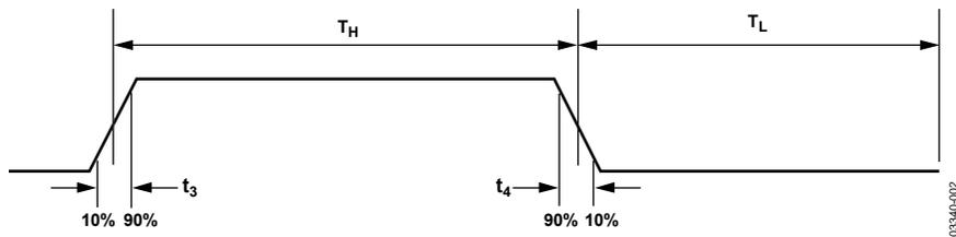
Figure 2. PWM Output Nominal Timing Diagram (25°C)
