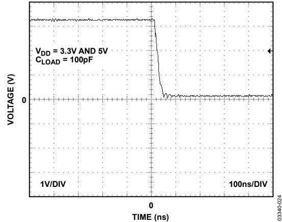
Figure 10. TMP05 Output Fall Time at 25°C
