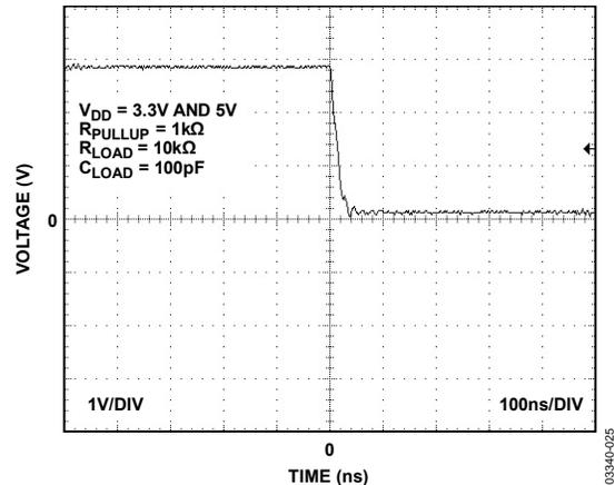
Figure 11. TMP06 Output Fall Time at 25°C
