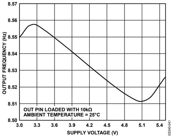
Figure 7. PWM Output Frequency vs. Supply Voltage
