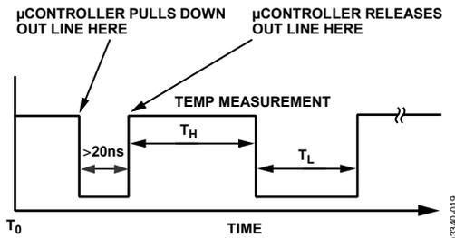
Figure 22. TMP05/TMP06 One Shot OUT Pin Signal
