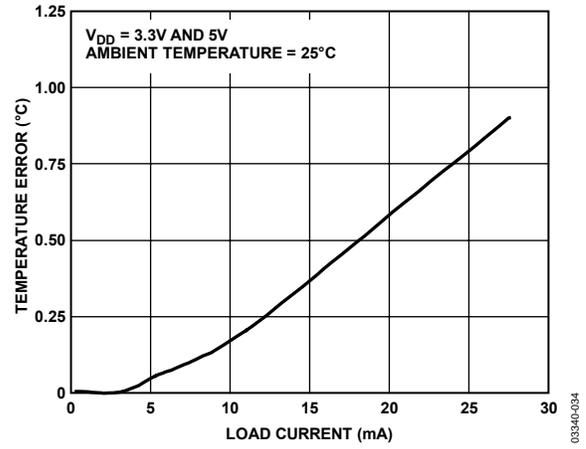
Figure 19. TMP05 Temperature Error vs. Load Current
