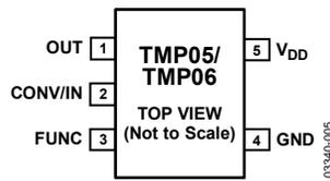
Figure 5. Pin Configuration
