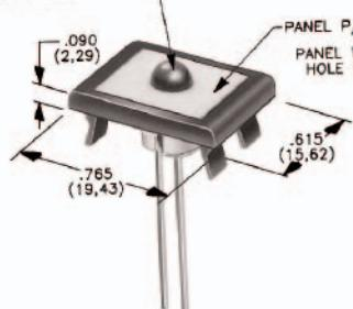
Above frames (part nos. 432XXXXXX) are also available with insert which accepts LED for indicator light assembly. Order insert separately from frame. Blank insert panel (without hole for LED) also available. **LED not included.**
