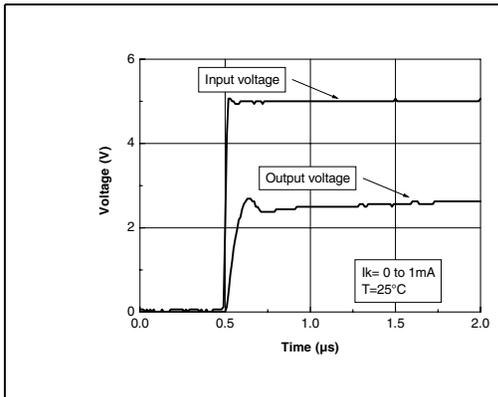
Figure 14. Pulse response at  $I_k = 1 \text{ mA}$
