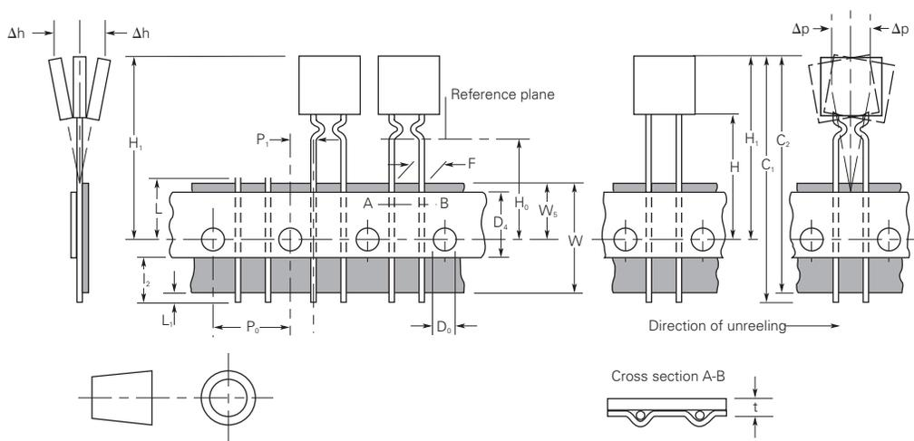
**Figure T23 Reel Dimensions for TRF Devices**
