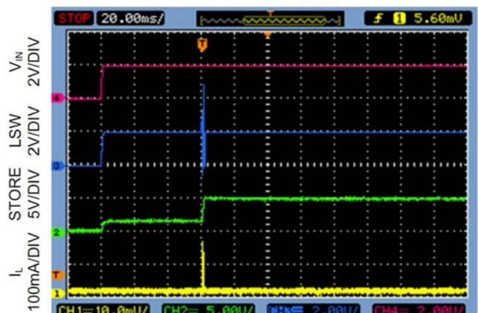
Startup : Circuit A with R_{IN}=10\Omega V_{IN}=2V , STORE=5V, I_{STORE}=0.5\mu A
