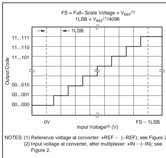
Figure 14. Ideal Input Voltages and Output Codes
