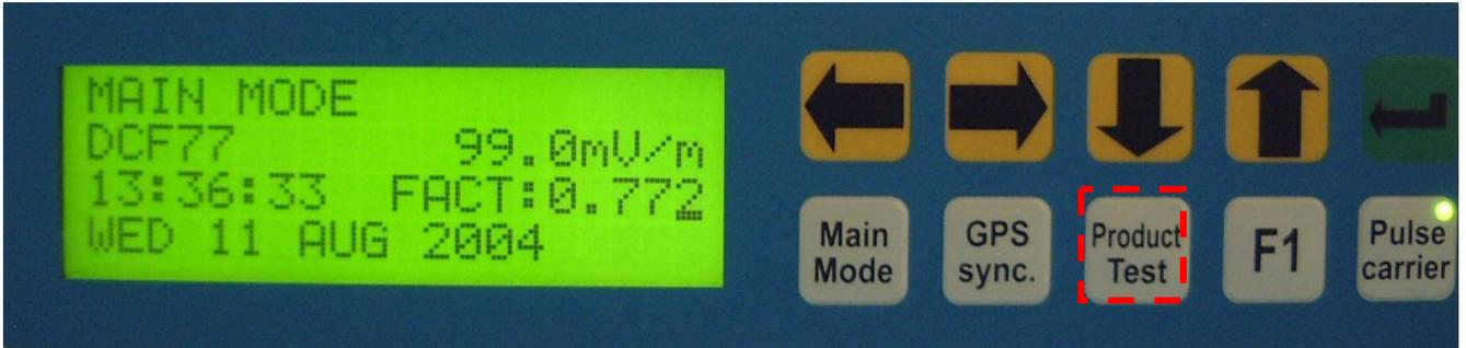
To activate the PRODUCTION TEST MODE, the button PRODUCT TEST button must be pushed.
