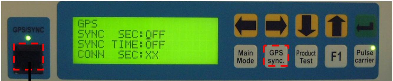
To start the GPS SYNC., push “GPS SYNC” button and connect the C-MAX “GPS100” unit by using the RJ45 GPS/SYNC. connector at the left side of the front panel.
