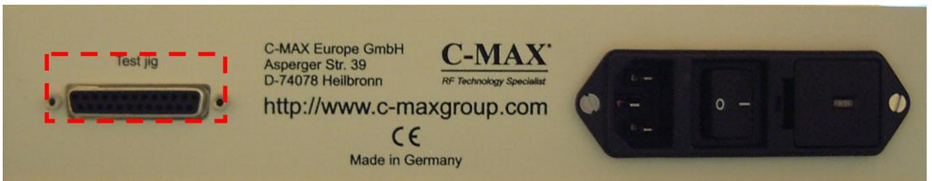
The test jig must be connected to the SUB25 parallel connector at the back side of the TSG800.
