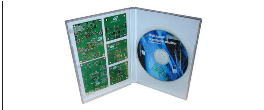
Figure 29. Evaluation kit for high-speed op-amps
