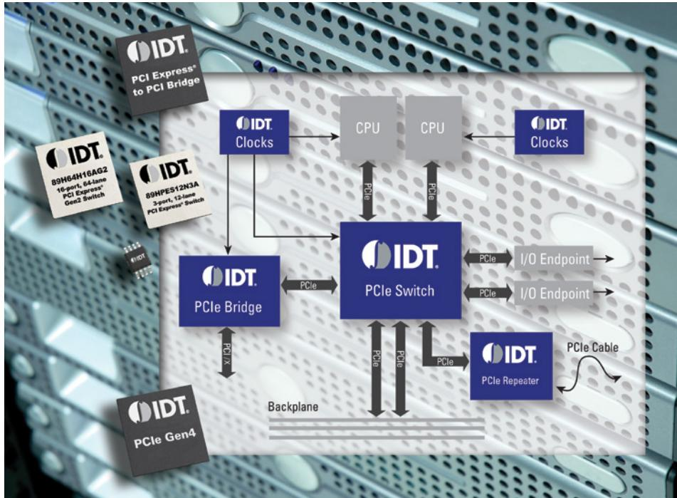
PCI Express® (PCIe®) is globally recognized as the general purpose I/O that unifies the component interconnect across many applications including desktop computing, servers, workstations, storage, networking, enterprise router, industrial test and control equipment, defense, aerospace and many more.
