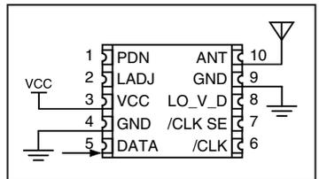
Figure 2: Test / Basic Application Circuit
