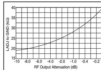
Figure 3: Level Adjust Attenuation
