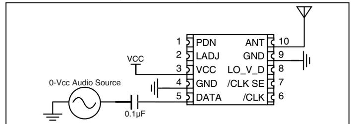
Figure 10: AC Coupling An Audio Source
