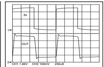
Figure 4: Square-Wave Modulation Linearity
