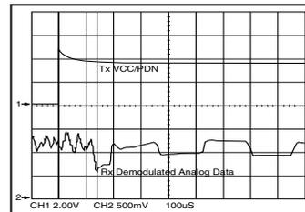
Figure 5: Tx Powerup to Valid Rx Analog
