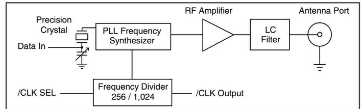
Figure 8: ES Series Transmitter Block Diagram
