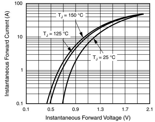
Figure 4. Typical Instantaneous Forward Characteristics Per Diode
